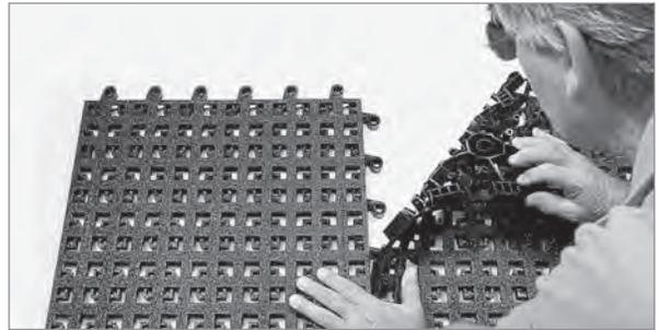
**Step 2 (b).** ErgoDeck is designed for easy, onsite customization. The tiles can be cut every 3" and still connect. Although, the tiles and ramps can be cut with an industrial shears, if you have multiple tiles to modify, we recommend the use of a band saw or a Skil® saw. These will also insure a straight cut.
