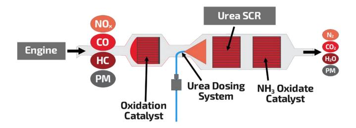
Most diesel pickups, trucks and SUVs that are a year model 2010 or newer have the SCR system. Several truck and engine manufacturers choose SCR as their leading technology choice because it allows them to meet the EPA's 2010 diesel emission standards for heavy-duty trucks.
