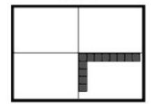
Starting with one quadrant, install a row of full tiles along both reference lines (see **Figure 4**). First apply the adhesive using a paint roller. Next, place the tiles along the reference lines applying firm pressure with the palm of your hand to ensure good contact with the adhesive. Tiles should be placed snug against the adjacent tiles and their edges accurately aligned with one another.
